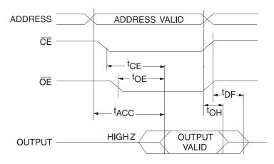
Notes: 1.  $\overline{\text{CE}}$  may be delayed up to  $t_{\text{ACC}}$  -  $t_{\text{CE}}$  after the address transition without impact on  $t_{\text{ACC}}$ .
