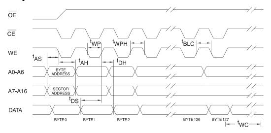
Notes: 1. A7 through A16 must specify the sector address during each high to low transition of  $\overline{\text{WE}}$  (or  $\overline{\text{CE}}$ ).
