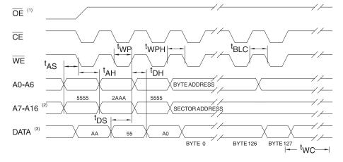
Notes: 1. A7 through A16 must specify the sector address during each high to low transition of WE (or CE) after the software code has been entered.
