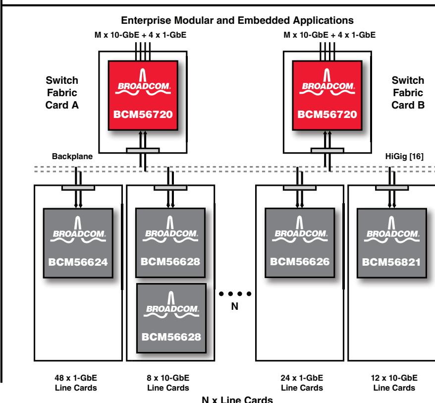
Note1: HiGig/10-GbE ports can drive connectors, backplanes or CX-4, and iPass cables directly, allowing physical switch device to be located anywhere in the system.
